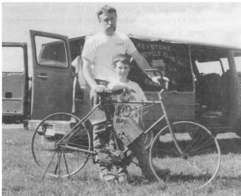
Brian Keating and his son, Nick, display their 1902 Keating motorcycle at Oley, PA. This machine, manufactured in Middletown, CT, featured a vaporizer located directly underneath the gas tank instead of a carbureter. The engine is a stressed member of the frame.
