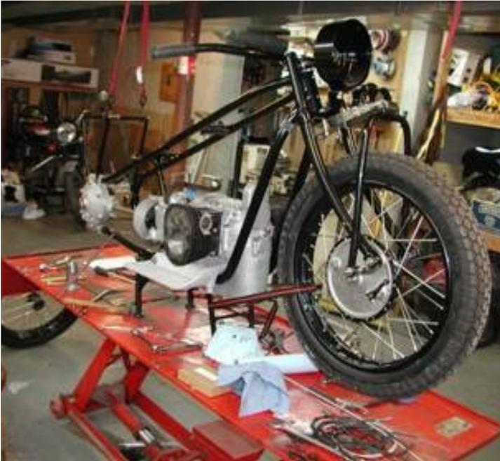
Late in 2009, I was able to trade the R11 brake parts and drive hub for a correct R62 brake assembly. Here is what the correct driveshaft, rear brake and final drive cover look like.
