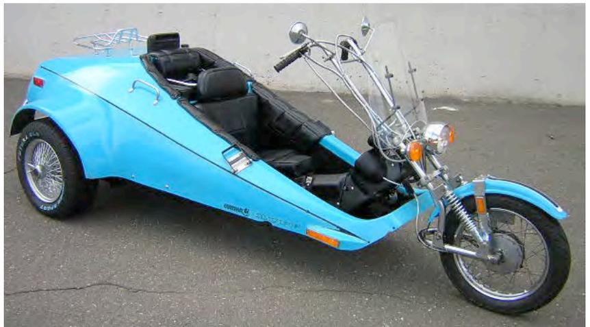
This machine was originally designed to have a VW Super Beetle motor in it (they still will bolt right up), but VW raised the price, so Rupp went to Kohler for the cheaper 340cc 2-stroke snowmobile motor and tranny. Tranny is a centrifugal clutch. These motors failed when run steadily at high RPMs. They also 'sploded when the injector belt failed or when it was too hot out.
